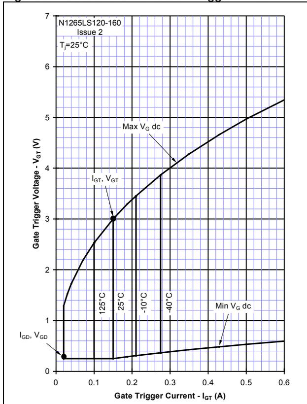
Figure 4 - Gate characteristics - Power curves
